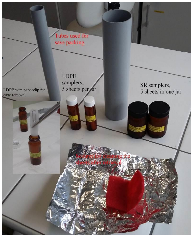
Figure 4: Plastic tubes containing scourer, jars/vials with samplers, each jar/vial labelled with “aqua-gaps FW” (FW – freshwater), type, and a sequence number
