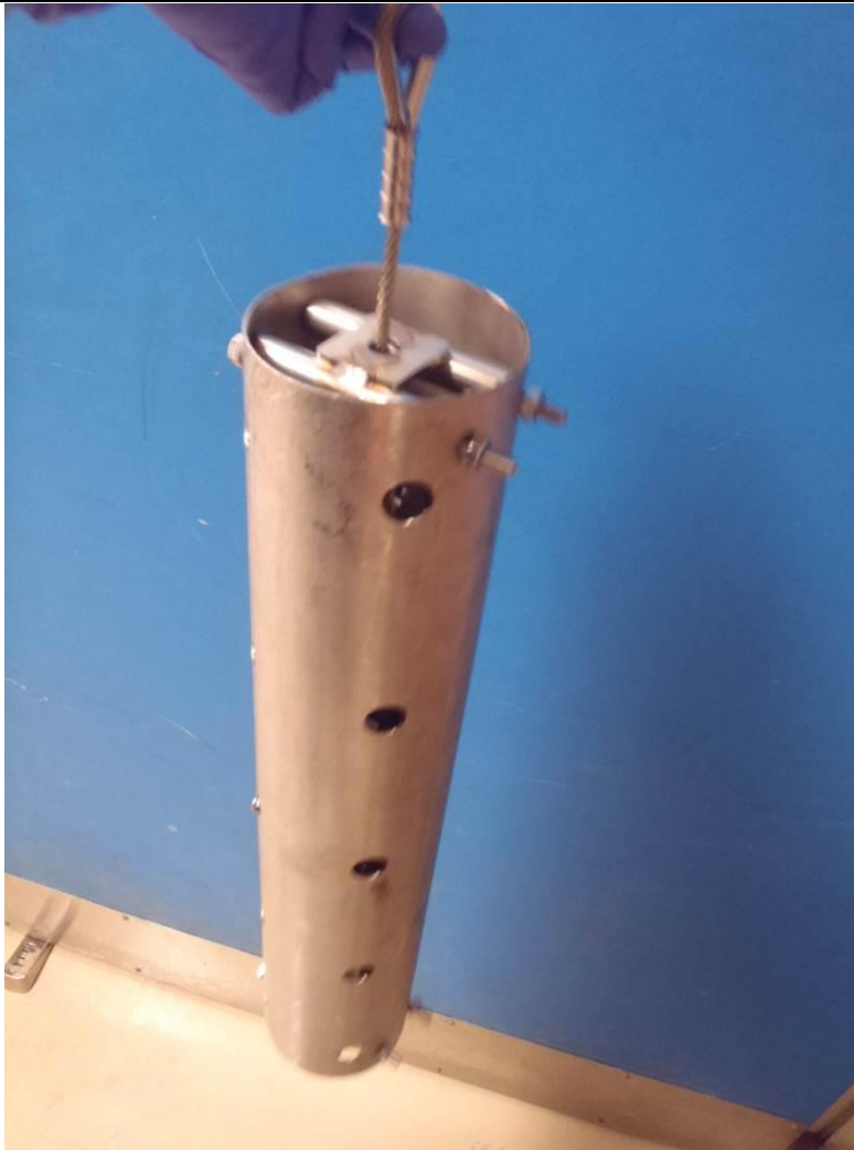
Figure 8: Bolts through shroud and holder – ready for deployment.
