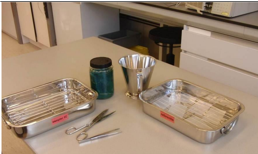
Figure 5: Materials especially required for retrieval of samplers. Please also bring along gloves, tools for removing nuts/bolts, thermometer/conductivity or salinity meter, the original jars from deployment for sampler storage, and clean lab tissues.
