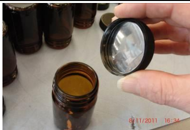
Note stainless steel lining easily falls out
