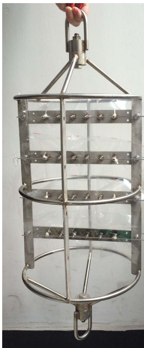
Figure 1 Aqua-gaps open sampling cage with 4 sample holders.
