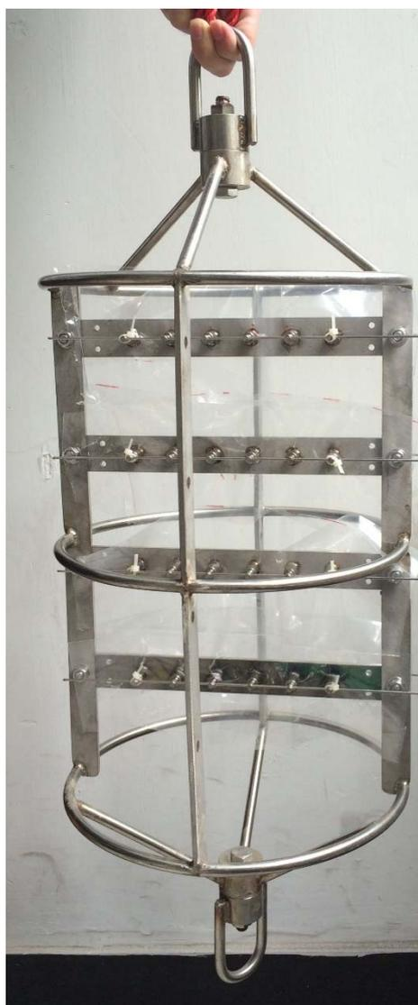
**Figure 1** Aqua-gaps open sampling cage with 4 sample holders.
