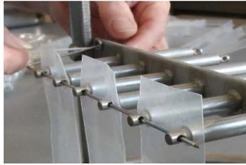
Feed the cable tie through the ring a hole in the holder
