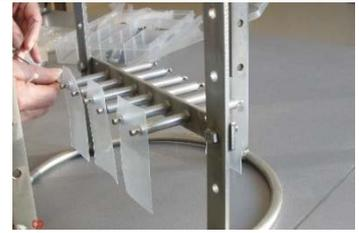
Feed the fixing rod through the holes on the stems
